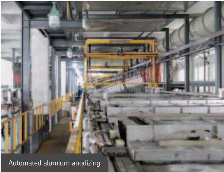
Automated aluminium anodizing
